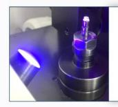
UV light is used for diamond fixing.
